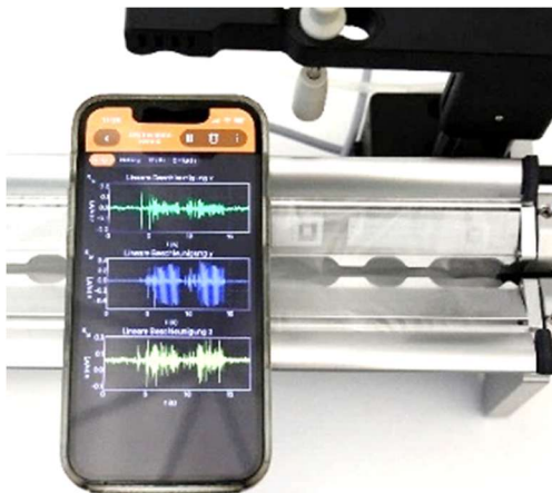
Fig. 2: Smartphone placed on the bag holder and running the phyphox app during data recording.
